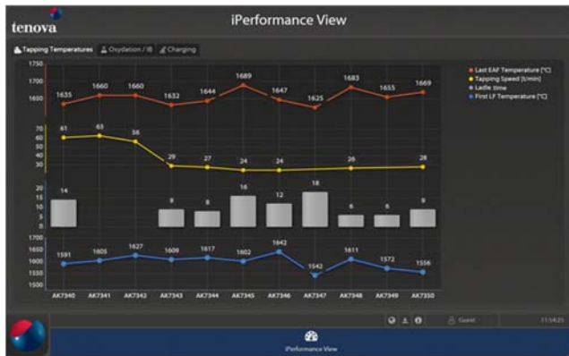
Figure 10: Data Mining and Report. Tapping parameters trend and statistic.
